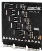
Module that easily fits into the **MC160** control board for operation with sound and light buzzer.
