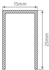
**MPV216** Gutter 25mm high and 15mm wide.
