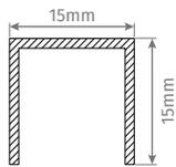
**MPV217** Gutter 15mm high and 15mm wide.
