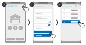
On your device's control page, click the *Edit* icon. On the editing page, click *Diagnostics*. You can test the control board using the buttons and check statuses in the list.
