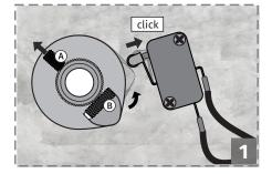
2 Loose the screw **A** opening micro (right ring) and adjust the ring until you hear the micro click. Turn to tighten the screw.
