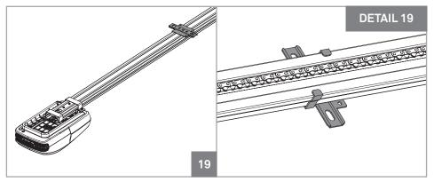
**03** • Place celling rail 's fixation plate roughly halfway through the steel rail as visible in the pictures above.
