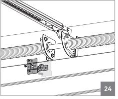
**06** • Attach the plates to the top of the door panel. The rods must be centered horizontally with the panel so that it stays aligned with the rail. It should also be to fixed as higher as possible (picture 24).
