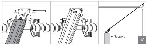
**02** • Fasten the rail in the fixation plate already attached. To facilitate the task, you can do it with the rail inclined (motor on the floor / support) which facilitates the installation since you only have to handle the area of rail to be fixed.
