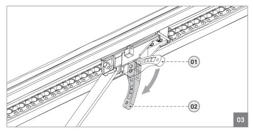
Position 01 • Motor locked Position 02 • Motor unlocked
