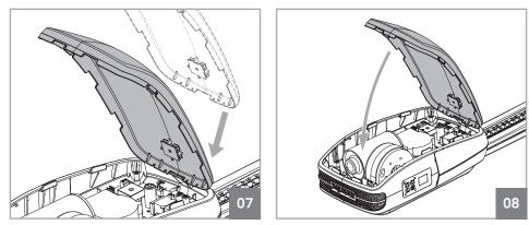
To replace the cover you must first fit the back as shown in the figure 07. Then simply turn down the cover and fit the front pressing down. The fittings will automatically secure the cover.
