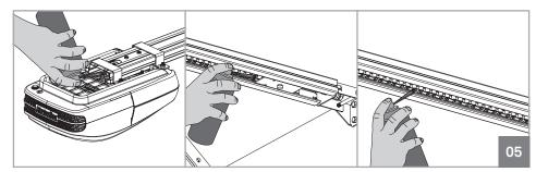
The only maintenance required is lubricating the automatism and rail motion axes. The pinions at both ends of the rails as well as their supporting bearings and chain should be lubricated at least once every year.
