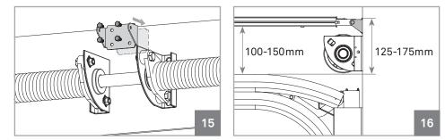
**01** • Attach the rail's support plate to the lintel, as visible in the image 15. In the image 16 if can be seen the distance to keep between the gate rail and support plate's upper part (125-175mm).
