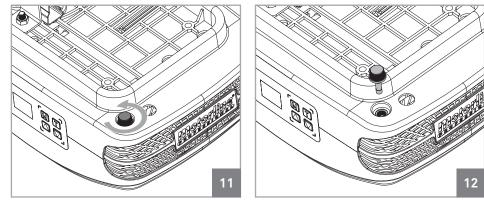
• To replace the fuse, first loosen it as visible in the image 11. Then just pull to remove it (image 12). Repeat the same steps in reverse order to put a new fuse. The operator uses a 250V 2.5A.
