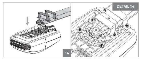
**02** • The aluminum rail and automatism attachment must be made using the plates and M6 nuts and as shown above. Tighten 4 screws, leaving the two in the front free.
