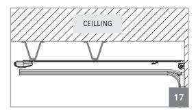
← Note • If you are unable to fix the rail to the ceiling for not respecting the measures above, there should be created a solid structure to be able to fix the motor in correct measurements. This structure may be fixed to the ceiling as a visible on the image 17.
