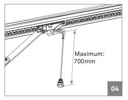
$\leftarrow$  Together with the automatism it is also provided a string to apply on the unlock lever, which makes it even a more practical and comfortable process.
