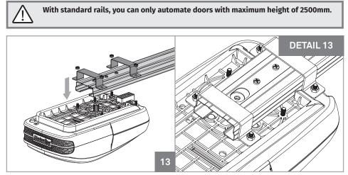
**01** • The steel rail and automatism attachment must be made using the plates and M6 nuts as shown above. Fasten 4 screws, leaving the two in the middle free.
