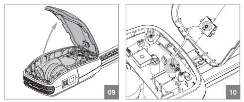
• To replace the LED board you must open the top cover and detach the wire of the LED from the control board. Loosen the screw which secures the LED board to the top cover and remove it. Now just put the new LED board, screw it, fit the wire in the control board and close back the cover on the motor.
