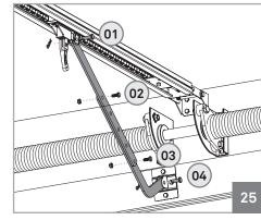
**07** • Now attach the two connecting rods between the trolley and the panel's upper plate.
