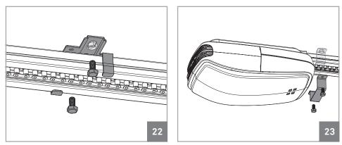
**05** • After rising the rail and mark the holes, you should fix the plate with screws. After that, you should use bracket to reinforce the attachment, this time near the motor (image 23).
