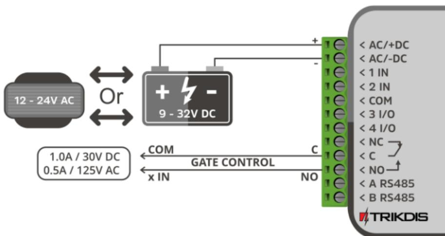
Find which contacts you need to connect to *GV17* relay contacts in the manual of the device that you wish to control. Usually these contacts are a certain input (x IN) and common terminal (COM).
