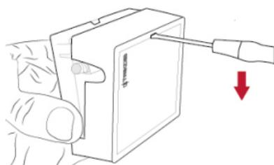
2. Take out the PCB board from the casing. Fix the casing to chosen place with self-tapping screws.
