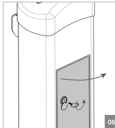
**01•** Open the door using the key supplied with the barrier. Rotate the key to unlock the door and pull it towards outside. On the interior, you will have access to the unlocking system.
