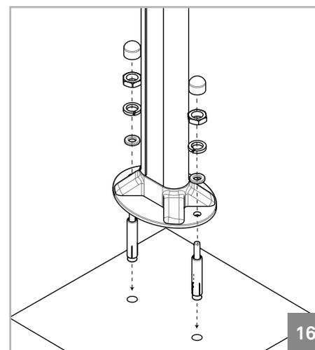
When the position of the boom's support is defined, you can fix it to the ground. Make two holes on the fixing ground, and place the screws supplied. Align the support holes with those same screws and fasten the support using the nuts.
