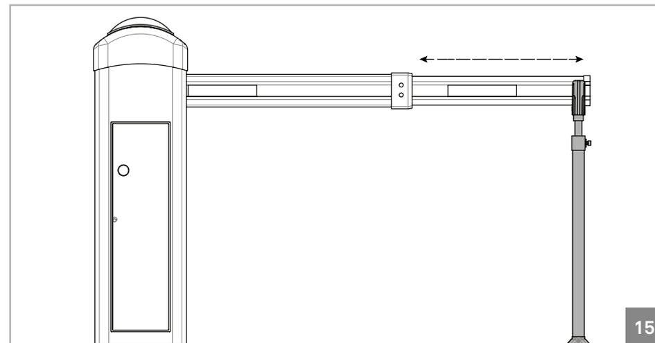
After assembling the boom, you must define the length of it so that you can fix the boom support, as visible on the image above. When the boom's length is decided, fix it with the two small screws situated at the end of the fix part of the boom.
